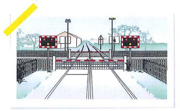
These have warning lights and alarms. Two barriers cover the whole road and the alarm stops once the barriers are lowered.
